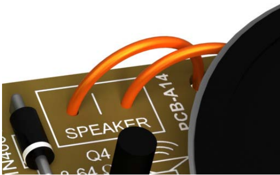
◀ Loudspeaker wired to the board.
