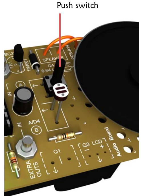
▲ A view of the GENIE Audio Kit, showing the push switch.
