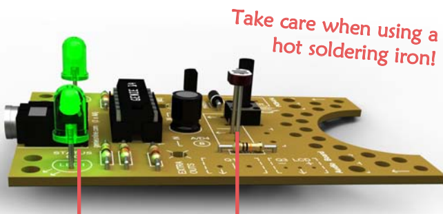
The LDR (not supplied) and LEDs are shown mounted above the base of the printed circuit board. This is optional for single-panel designs, but is recommended for double-panel designs (so that the components are not obscured by the upper panel).
